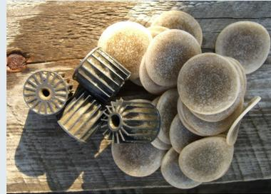
For comparison: clogged carrier (left) & chip-type carrier (right).
