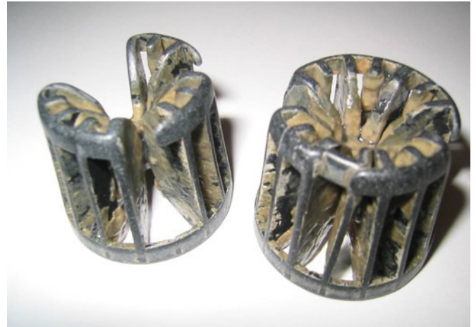
Fig. 2: Carriers damaged by too high kinetic energy
