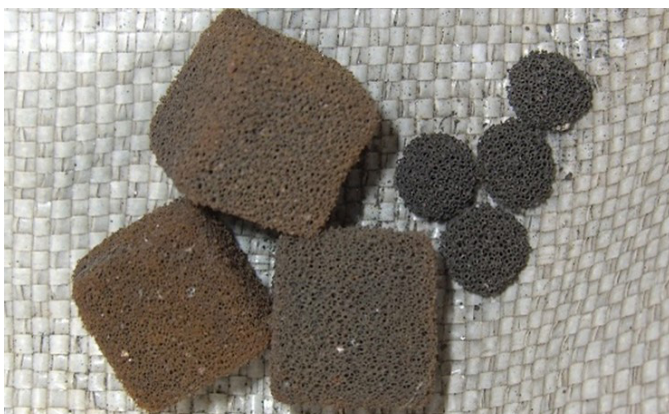
Fig. 1: Foam-type carrier: virgin material (left) and abraded material (right)
