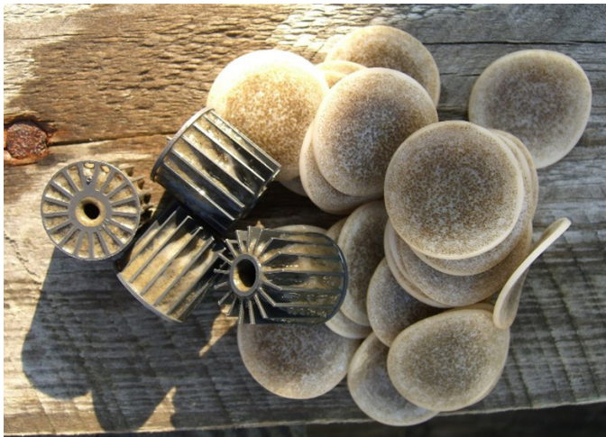
Fig. 4: For comparison: clogged carrier (left) and chip-type carrier (right)
