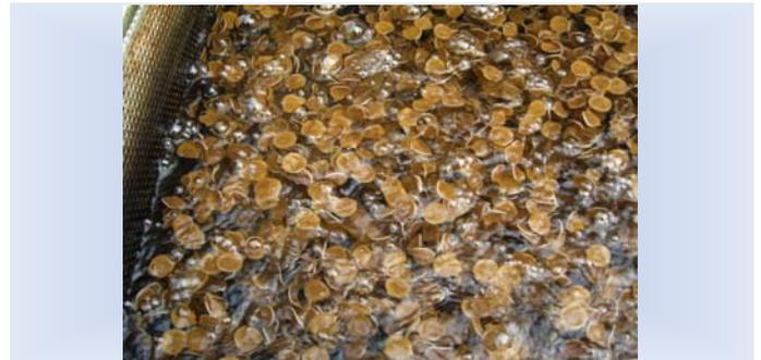
Fig 2: Mutag BioChip™ nitrification in the RAS of a sturgeon farm
