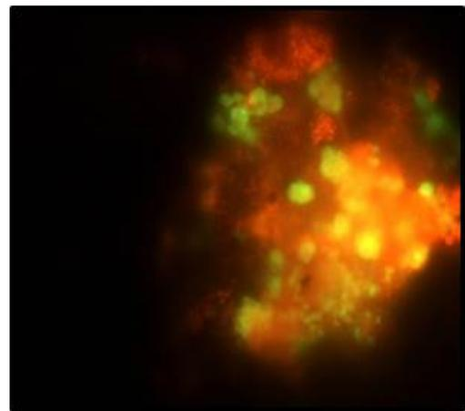
Fig. 4: Ammonium-oxidizing (red) and nitrite-oxidizing bacteria (green) in a pore of the Mutag BioChip™ carrier.
