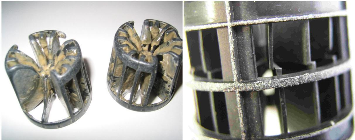
A flexible and simultaneously highly wear-resistant material is more likely to be used. Sponge-type carriers are flexible indeed but they show signs of abrasion already after a short operating period. Contrary to this, highly fine-porous chip-type carriers (Mutag BioChip™) are offering all of the desired characteristics such as a high wear resistance, flexibility, virgin material and many more.
