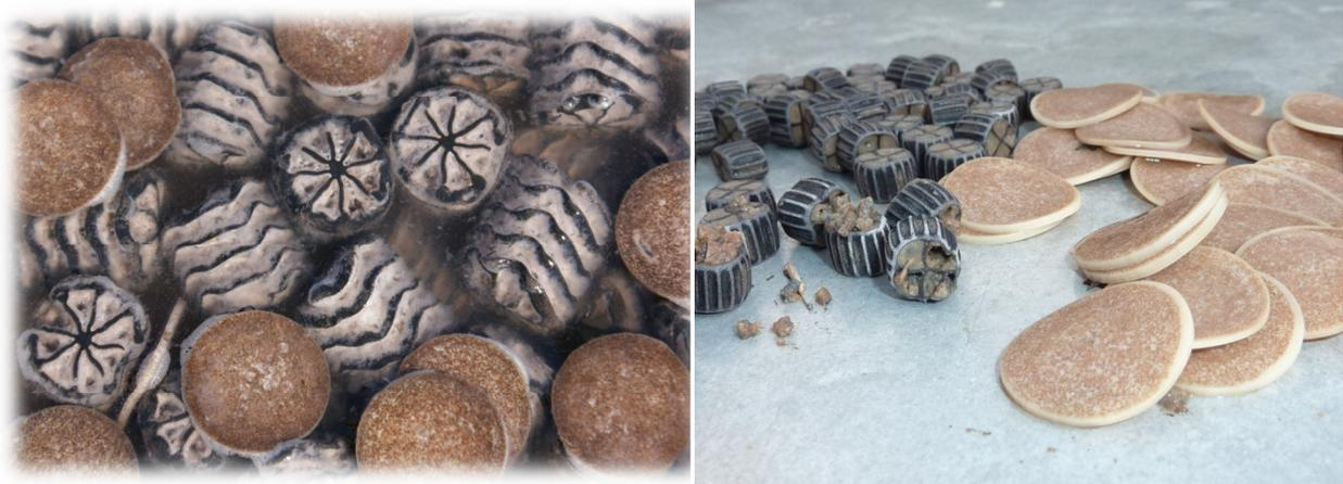
The pictures above show several carriers which have been applied together with the disk-shaped carrier (Mutag BioChip™) in the same wastewater. Neither a clogging nor an abrasion of the chips can be observed.
